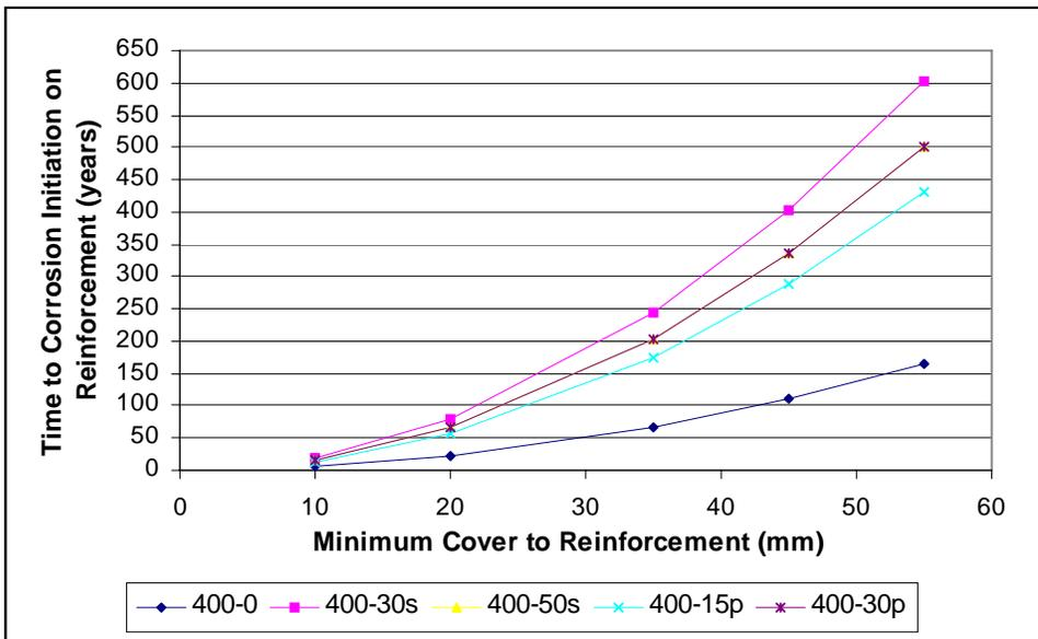
Figure 2 Time to corrosion initiation for a given cover, concrete with 400 kg/m<sup>3</sup> binder content, notional surface concentration of 1.2% and chloride threshold value of 1.0%
