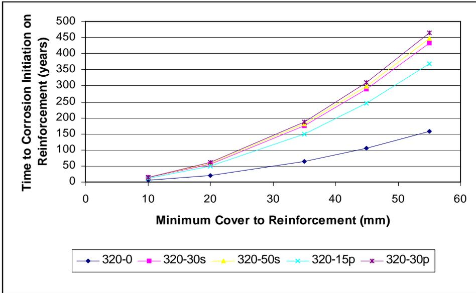
Figure 1 Time to corrosion initiation for a given cover, concrete with 320 kg/m<sup>3</sup> binder content, notional surface concentration of 1.2% and chloride threshold value of 1.0%
